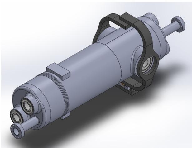
Figure 2: QWR Cavity and Liquid Helium Jacket.
