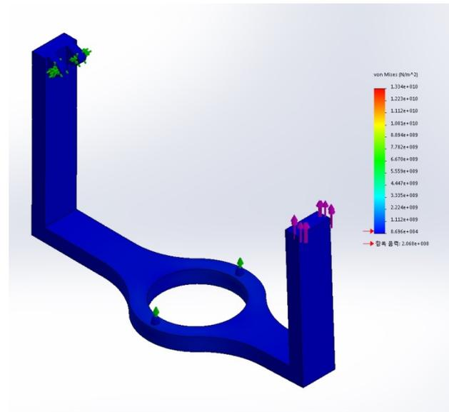
Figure 3: Von-Mises Stress of Tuner Lever Arm.
