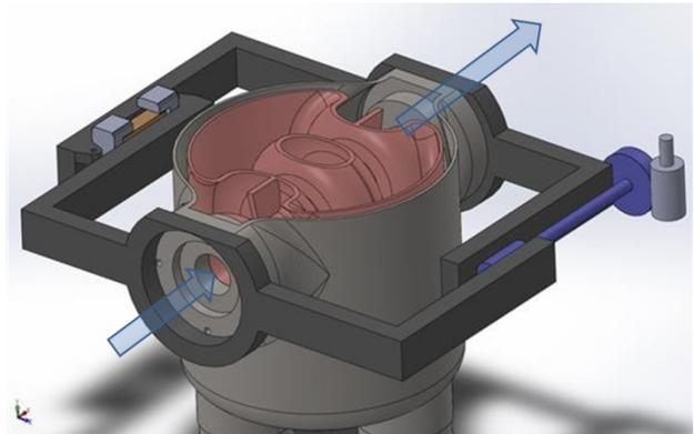
Figure 1: Layout of Slow Tuner for QWR Cavity.
