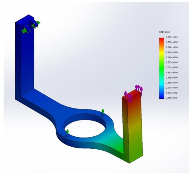
Figure 4: Von-Mises Strain of Tuner Lever Arm.
