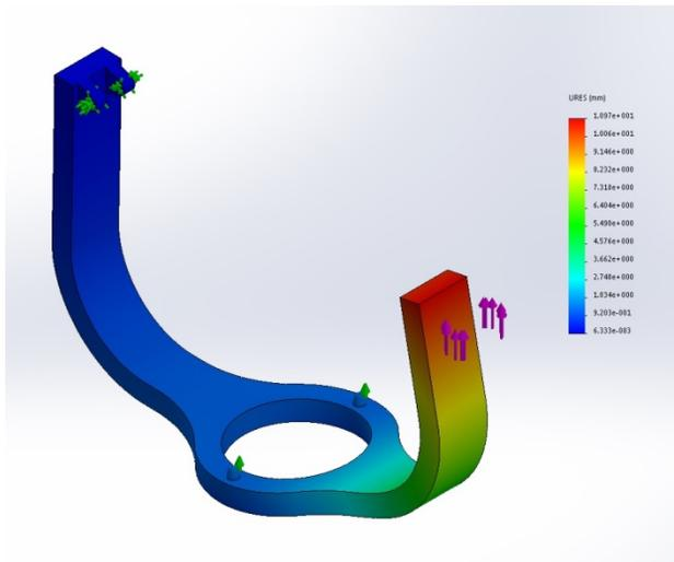
Figure 6: Von-Mises Strain of Modified Lever Arm.
