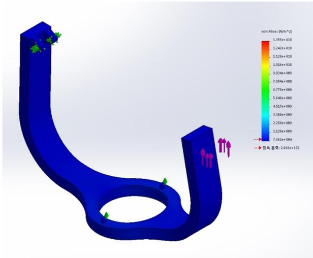
Figure 5: Von-Mises Stress of Modified Lever Arm.
