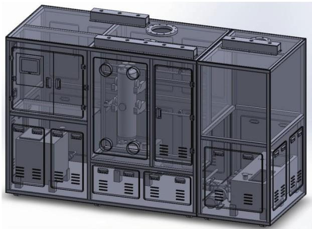
Figure 2: Perspective view of BCP cabinet for RISP cavities
