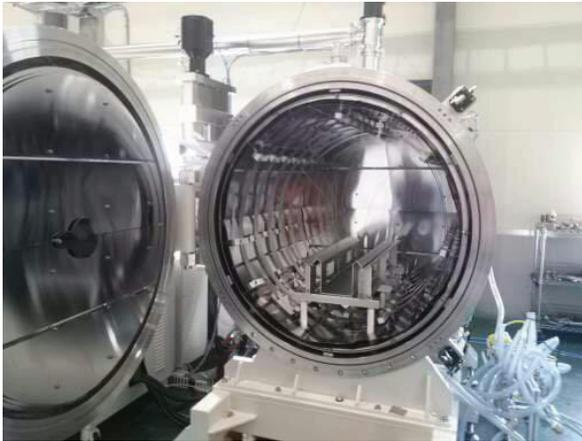
Figure 5: High vacuum furnace of RISP
