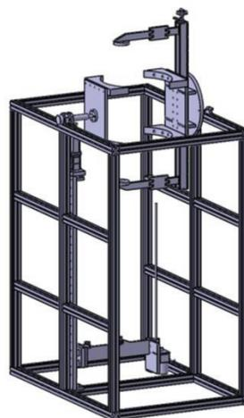
Figure 3: 3-dimensional model of high pressure water rinse cabinet
