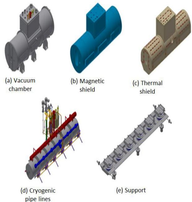
Figure 1: Components of SSR2 cryomodule
