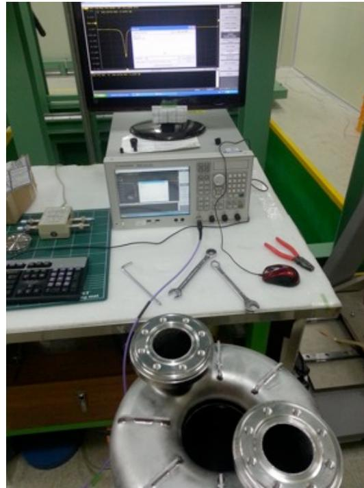
Figure 7: Clamp up of the HWR.
