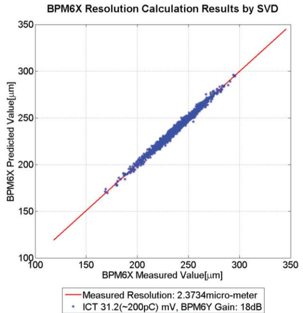
Figure 8: Achieved measuring resolution in horizontal plane using SVD calculation method.
