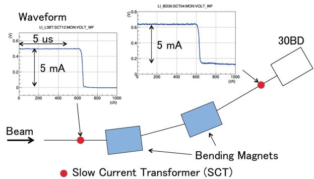
Figure 3: Beam transmission to the 30BD.
