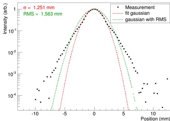
Figure 5: Transverse beam profile at the ACS exit with peak current of 25 mA and beam energy of 400 MeV. the red and green dotted lines are same as those of in Fig. 4.
