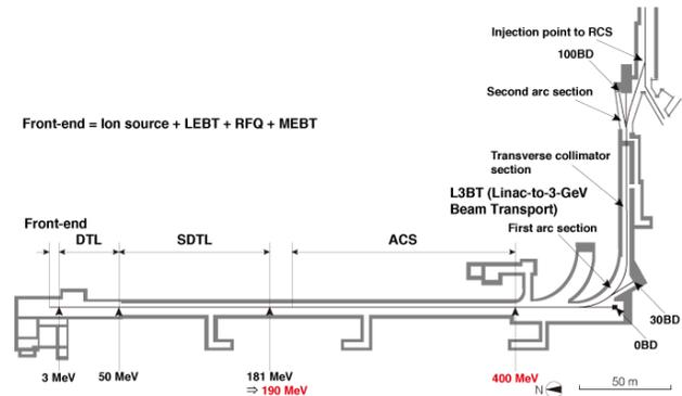
Figure 1: Outline of the J-PARC linac. In the initial stage, the linac had been operated at 181 MeV by the installation of IS to SDTL on the beam line as shown in black character. The ACS accelerator was installed at second stage to extend the beam energy to 400 MeV (red).
