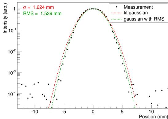
Figure 4: Transverse beam profile at the ACS entrance with peak current of 25 mA and beam energy of 191 MeV. Noise level is order of  $10^{-4}$ . A red dotted line shows the fitting results by Gaussian function, and a green one is a Gaussian function of which  $\sigma$  is RMS of the distribution.
