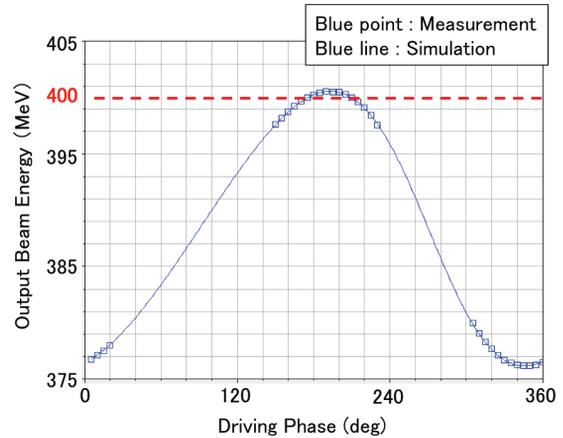
Figure 2: The phase scan curve of the last ACS cavity.
