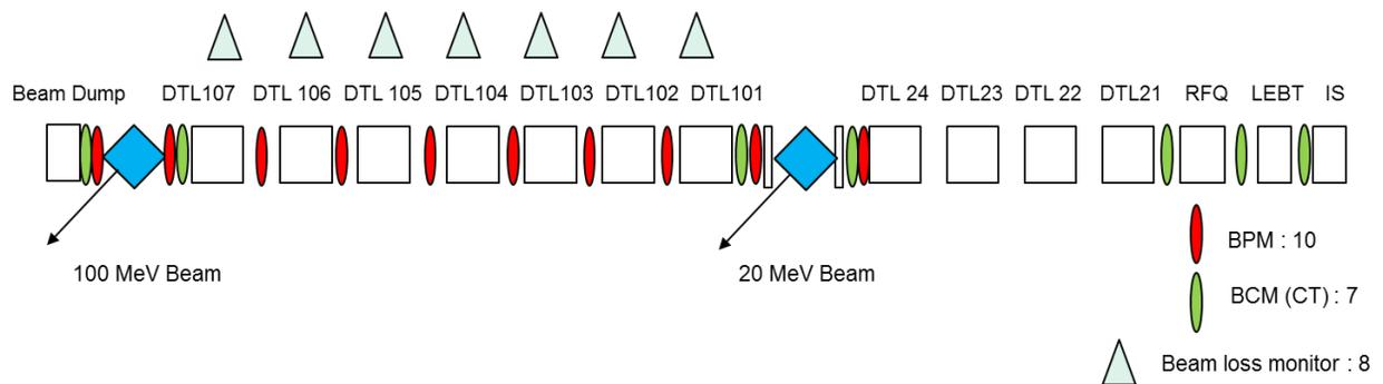
Figure 1: Layout of beam position monitors, beam current monitors and beam loss monitors along the linac.
