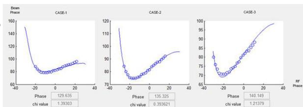
Figure 6: Comparison the artificial experimental data to the simulation results with different relative amplitudes ( $A/A_0 = 0.98, 1.0, 1.02$ ).
