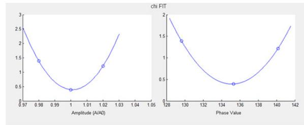
Figure 7: Determination of the RF amplitude (left) and phase (right) by using a quadratic fitting.
