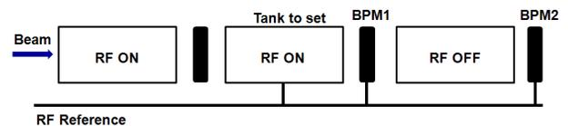
Figure 4: Schematic plot for beam phase measurement of a DTL tank by using BPM.
