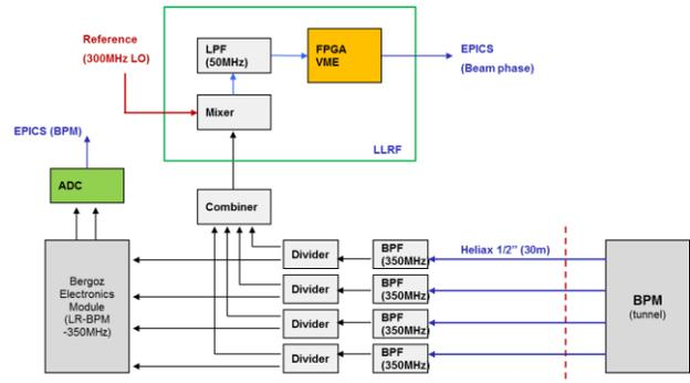
Figure 3: Data path of BPM signal for beam phase measurement
