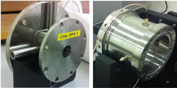
Figure 2: The fabricated linac BPM (left) and the beamline BPM (right).
