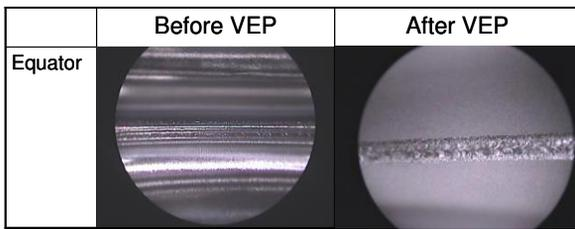
Figure 6: Images of inner surface of cavity (equator) before and after VEP observed with an endoscope.
