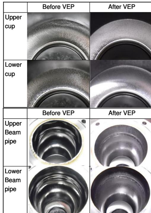
Figure 5: Images of inner surface of cavity (upper and lower cup, upper and lower beam pipe) before and after VEP observed with a digital camera.
