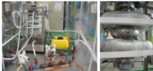
Figure 2: (Left) Picture of single-cell VEP system. (Right) Picture of single-cell cavity.
