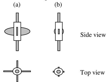
Figure 1: Schematic view of “i-cathode Ninja”<sup>®</sup>. (a) unfolded status. (b) retracted/folded status.
