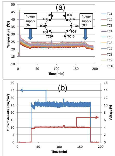
Figure 4: (a) Logged data of temperature of cavity. (b) Logged data of current density and voltage.
