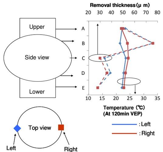
Figure 8: Relationship between temperature and removal thickness.
