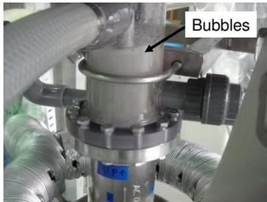
Figure 3: Picture of bubbles at upper side during VEP.
