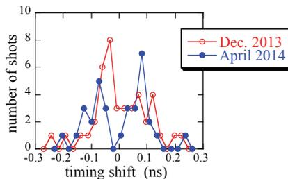
Figure 8; Time jittering (timing distribution) of the gate pulse at before and at after fixing the timing module.
