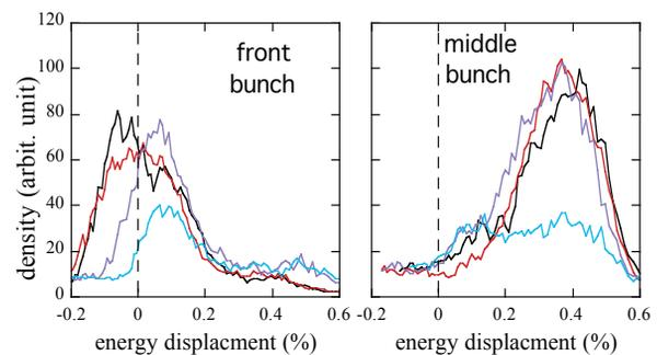
Figure 12: Shot-by-shot fluctuation of the energy profile. The horizontal axis is the displacement from the ring energy. A weak bunch had a larger energy spread.
