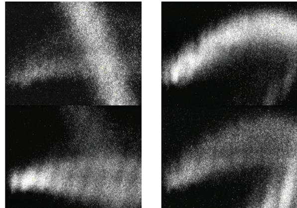
Figure 11: Synchrotron oscillation of a bunch. The vertical and the horizontal full scales are 0.32 ns and 0.6  $\mu$ s respectively. The front bunch (left two images) or the middle bunch (right two) were injected at the synchronous phase. The steep crossing lines were the light from the other bunch.
