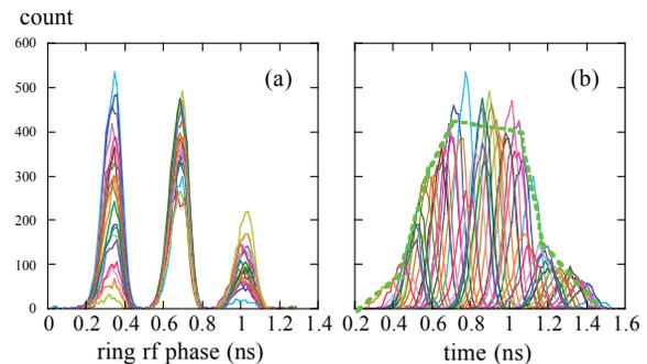
Figure 7: Linac bunch structure (a) and the effective pulse structure reconstructed with the correction of timing jitter.
