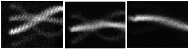
Figure 2: Typical dual-sweep streak camera images after the injection. The vertical axis is the ring rf phase with full scale of 1.27 ns. The horizontal axis is the revolutions in the ring with full scale of 0.123 ms.
