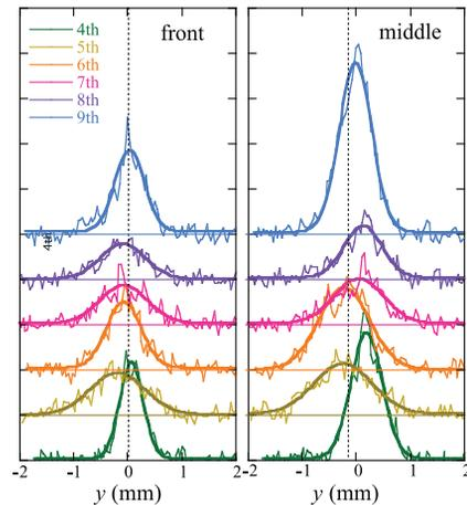
Figure 6: Vertical beam profiles of 6 turns of the front and the middle bunch. The profiles are fitted with Gaussian.
