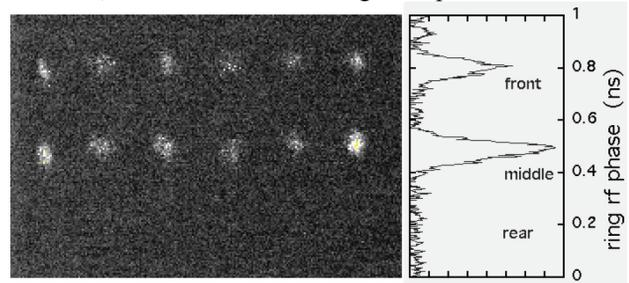
Figure 5: Dual Sweep streak camera image of the injected beam for 6 turns. The revolution period is 0.396  $\mu$ s.
