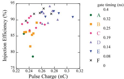
Figure 9: Injection efficiency for different bunch structure. The bunch structure was represented by the timing shift.
