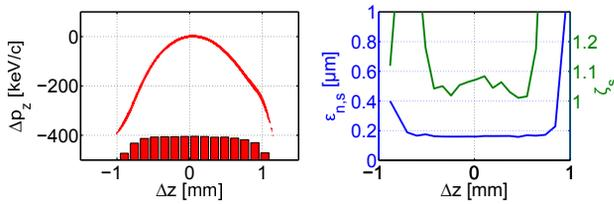
Figure 5: Longitudinal phase space and corresponding charge distribution of the 200 pC bunch (left), normalized slice emittance  $\epsilon_{n,s}$  and mismatch parameter  $\zeta_s$  (right) after the second TW structure ( $z = 12$  m and  $E = 130$  MeV).
