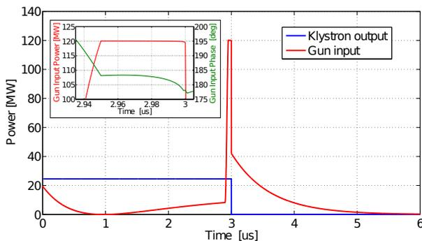
Figure 3: Rectangular RF pulse output from the klystron and corresponding RF input pulse to the gun after the BOC pulse compressor (20% waveguide losses accounted for). The inset provides a zoom of the 50 ns time interval for beam operation.
