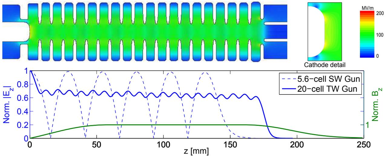
Figure 2: Magnitude of the electric field on a longitudinal slice of the TW gun normalized to 135 MV/m at the cathode (top), detail of the cathode region (top right), magnitude of the longitudinal electric field on-axis  $|E_z|$  and longitudinal magnetic field  $B_z$  of the gun solenoid (bottom). For comparison, the electric field profile of the SW gun is also plotted.
