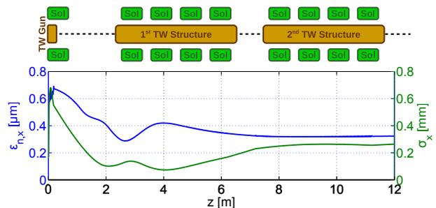
Figure 4: Normalized projected transverse emittance  $\epsilon_{n,x}$  and rms beamsize  $\sigma_x$  along the beamline sketched on top.
