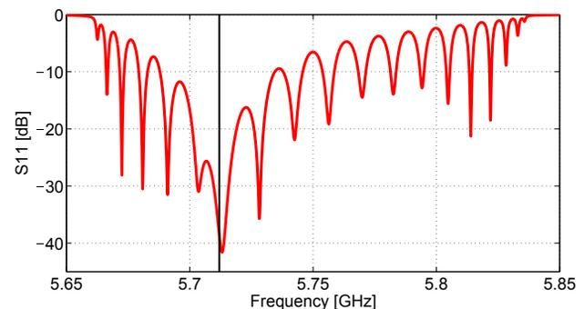
Figure 1: RF frequency spectrum of the TW gun of Fig. 2. The operating American C-band (5.712 GHz) is indicated.
