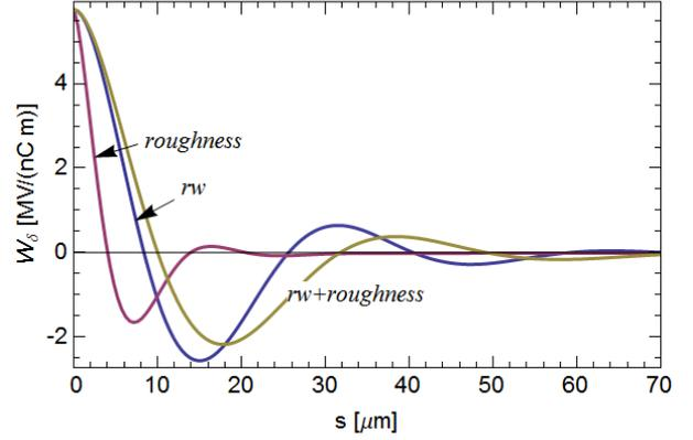
Figure 1: For round geometry, with radius  $a = 2.5$  mm: point charge wake  $W_\delta(s)$  for a pipe with resistance (blue), roughness (red), and both resistance and roughness (yellow). The roughness model assumes  $(y')_{rms} = 30$  mr.
