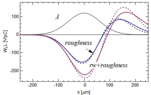
Figure 2: Bunch wake as obtained by ECHO (solid curves) and analytically (dashes) for test examples: (1) a lossless, corrugated pipe (blue), and (2) a lossy, corrugated pipe (red). The bunch shape  $\lambda$  is also shown, with the head to the left.
