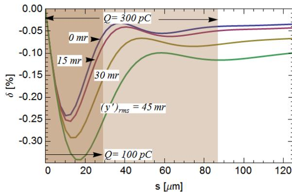
Figure 3: Flat geometry:  $W_\delta(s)$  (top) and relative induced voltage for uniform bunch,  $\delta_w(s)$  (bottom), considering resistance plus roughness, for  $(y')_{rms} = 0, 15, 30, 45$  mr.
