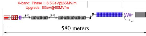
Figure 3: Layout of hard X-ray FEL at SINAP
