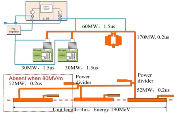
Figure 8: Layout of X-band RF microwave system
