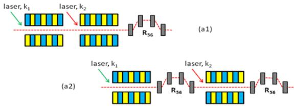
Figure 1: (color) layout of two schemes to generate THz density modulation in a relativistic electron beam.
