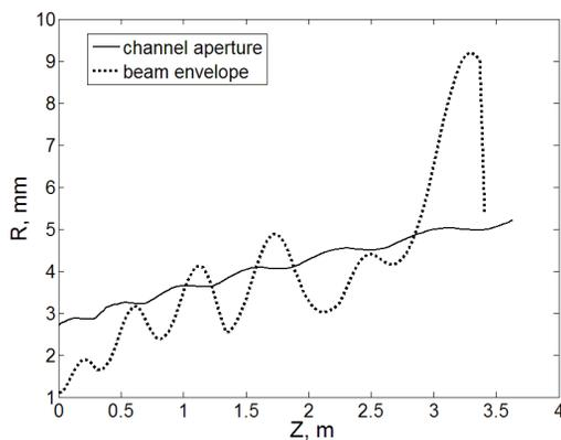
Figure 4: Beam envelope before correction
