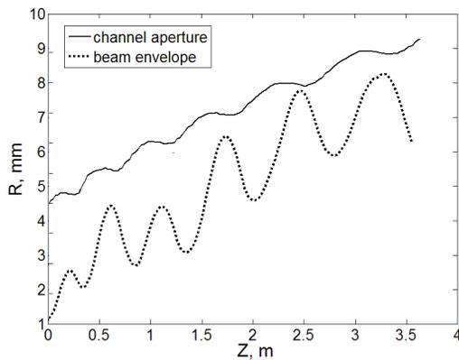
Figure 5: Beam envelope after correction
