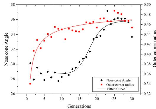
Figure 4: Parameter Values Variation: Nose-cone Angle and Outer Corner Radius.
