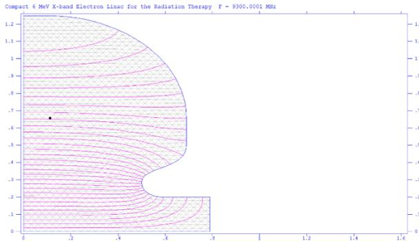
Figure 6: Half-cell of the Optimized RF cavity Single Cell.
