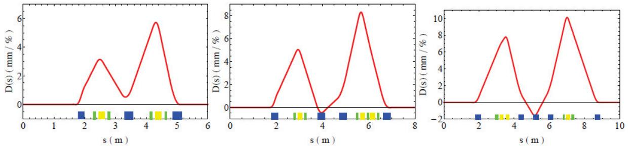
Figure 3: Transverse dispersion of the electron beam in the recirculation arcs of the S-DALINAC in the first, second and third recirculation (from left to right side). Dipole magnets are marked blue and quadrupoles yellow. The green areas mark possible positions for additional sextupole magnets which will be placed at positions with as high dispersion as possible..
