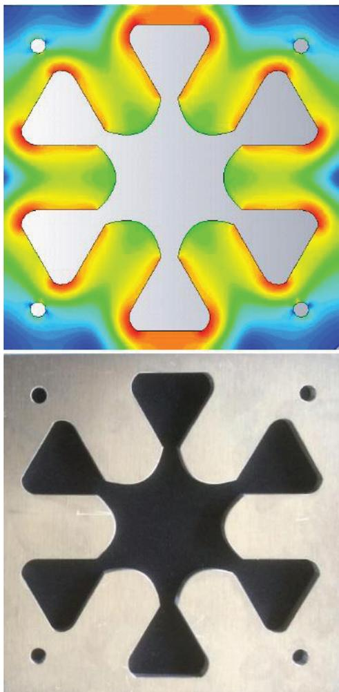
Figure 5: Simulated fields in the yoke (top) and photograph of a sheet (bottom) of the new sextupole. The sheets have a size of 20 cm x 20 cm.
