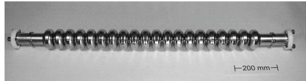
Figure 2: S-DALINAC 20 cell cavity. .
