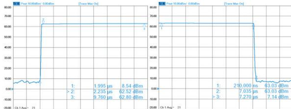
Figure 4: Rising and falling edges of 3.5 ms pulse, .10-90% rise time – 0.24 μs, fall time – 0.235 μs.
