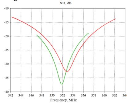
Figure 6: S11 parameters of 12:1 power combiner: green – calculated; red – measured.
