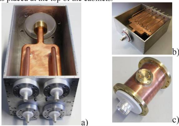
Figure 5: a: 4:1 final power combiner; b: 12:1 100 kW power combiner; c: bi-directional coupler.
