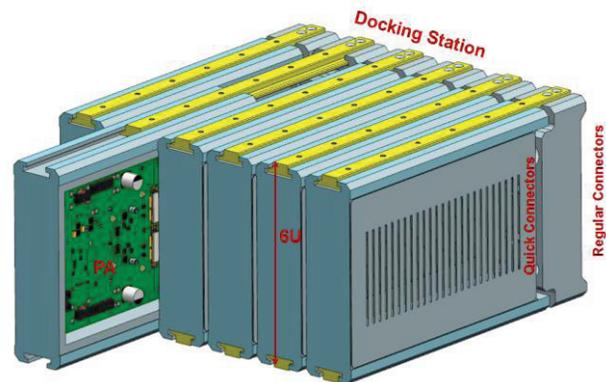
Figure 2: The general view of RF modules block with six modules and the docking station.
