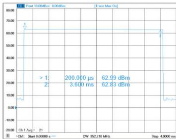
Figure 3: RF power stability. Power droop through pulse 0.13 dB.
