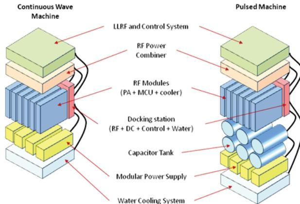
Figure 1: The general architecture of Siemens' solid-state amplifier.
