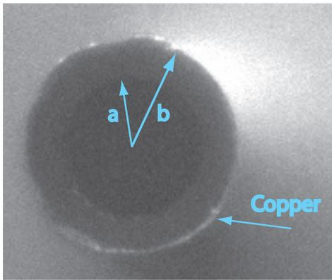
Figure 2: An image of one of the ends of a structure similar to the ones used in this experiment. The inner radius  $a$  is vacuum while the outer radius  $b$  is the structure diameter. In this case  $a = 200 \mu\text{m}$  and  $b = 300 \mu\text{m}$ . The reflective outer surface is the copper coating used to contain the mode, which is approximately  $20 \mu\text{m}$  thick.
