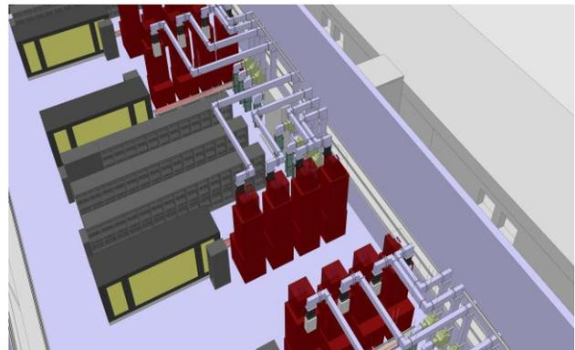
Figure 1: Preliminary typical layout in the RF gallery.
