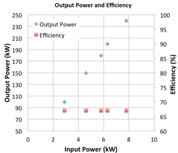
Figure 2: Measured data of a single tetrode under test. At 200 kW the anode voltage was 16 kV, screen grid and control grid voltages were 900 and -200 V respectively and the anode current was 18.7 A.
