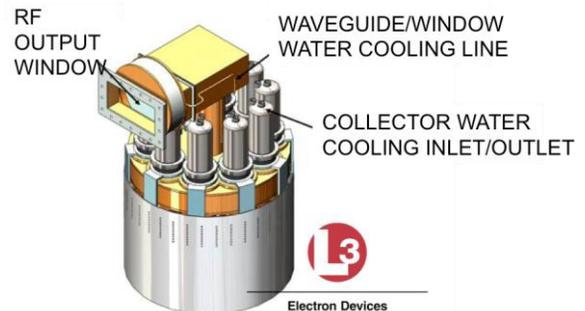
Figure 4: Possible configuration for a 1.2 MW multi-beam IOT under consideration. Courtesy of L-3 Electron Devices.
