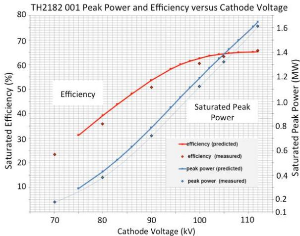
Figure 3: Saturated power and efficiency at saturated power as a function of high voltage. Note: This data was measured to satisfy CERN SPL parameters at 1.7 ms and a repetition rate of 50 Hz. The data is supplied courtesy of CERN and Thales Electron Devices.
