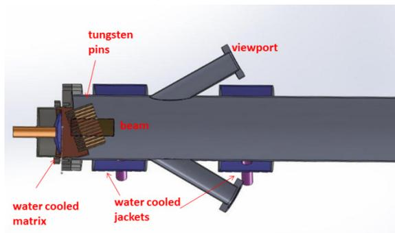
Figure 6: A schematic view of a pin beam dump
