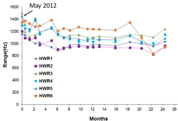
Figure 4: Tuning range of HV piezo tuners measured during the period over two years.
