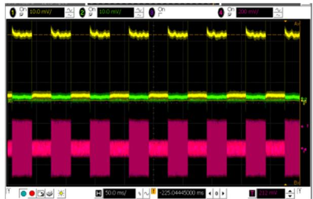
Figure 2: Screenshot of 250 kW operation at 50% duty cycle. The yellow, green and rose traces are forward power, reflected power and field pick up signals, respectively.
