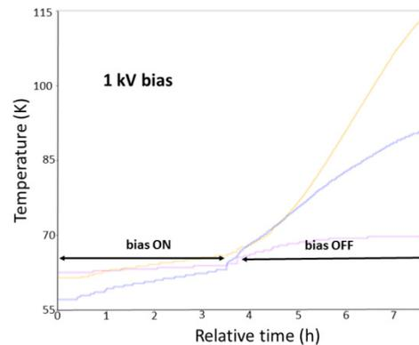
Figure 5: Effect of application of 1 kV bias on the coupler warming rates.
