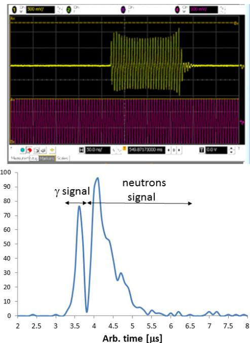
Figure 1: Layout of papers Top. A 160 ns beam pulse from the slow chopper. Pulse measured by BPM pick-ups. Bottom. A measured TOF neutrons spectrum generated with 4 MeV proton pulses on lithium target.
