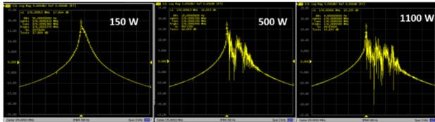
Figure 3: Resonance curves at several RF power values
