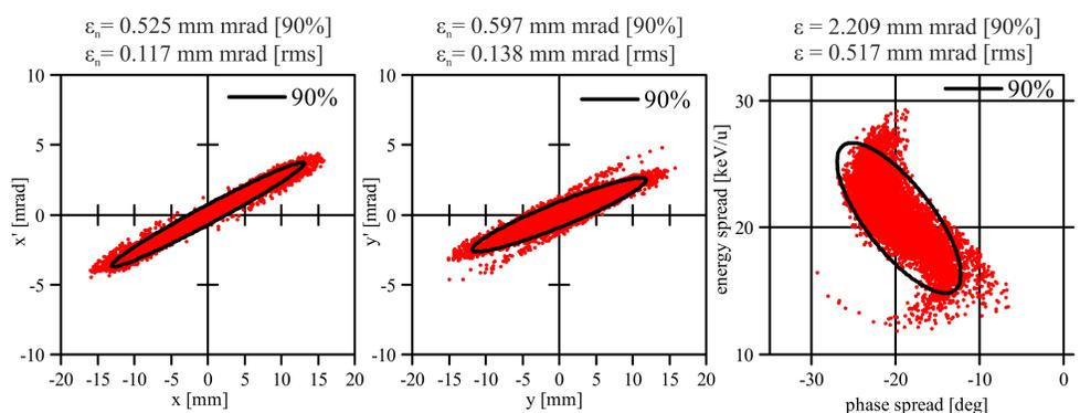
Figure 7: Output distributions of the IH-DTL with injection from the proposed MEBT.
