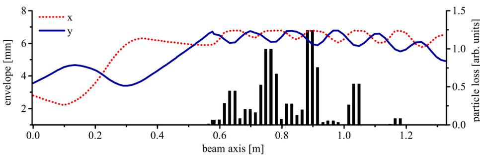
Figure 2: Loss profile of the current MEBT superlens for 20.75 mA  $U^{4+}$ .
