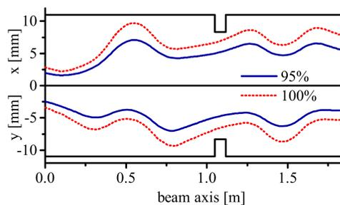
Figure 3: Transversal beam envelopes for the proposed MEBT section.
