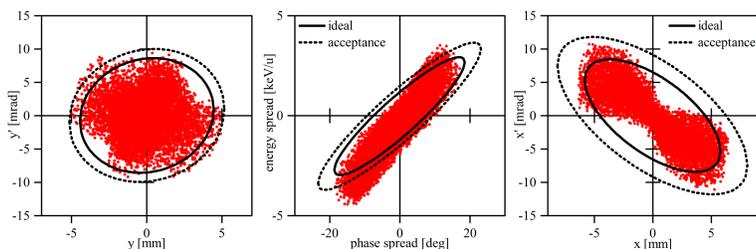
Figure 1: Output of the superlens for 20.75 mA  $U^{4+}$  compared to the acceptance of the IH-DTL.
