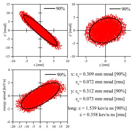
Figure 4: Output distributions of the proposed MEBT section.
