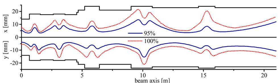
Figure 6: Transversal envelopes of the IH-DTL with injection from the proposed MEBT section.
