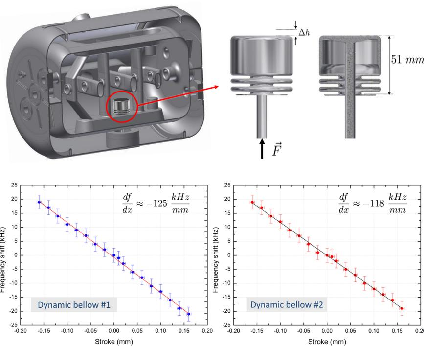
Figure 2: Measured frequency tuning range of the two dynamic bellow tuners of the sc 325 MHz CH-Cavity
