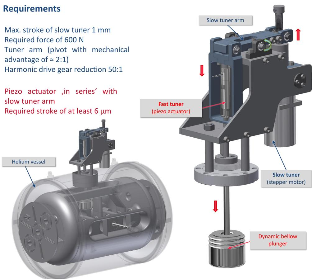
Figure 1: Piezo-based frequency tuner mounted on top of the helium vessel of the sc 325 MHz CH-Cavity (left) and complete frequency tuning system including the 3-cell dynamic bellow plunger (right)
