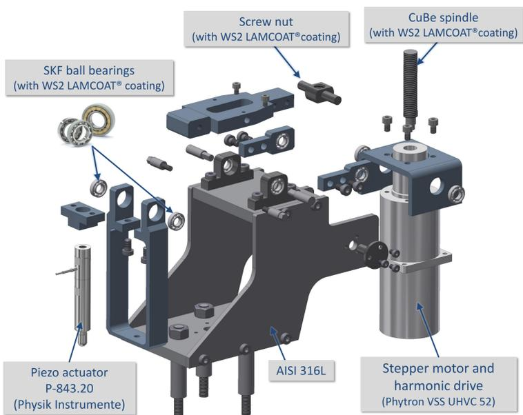
Figure 3: Main components of the frequency tuner drive system
