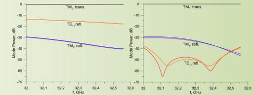
Efficiency of taper: left - 5 periods taper, right - 10 periods taper
