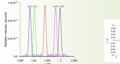
Spectrum of electron radiation with sharp edge pulse
