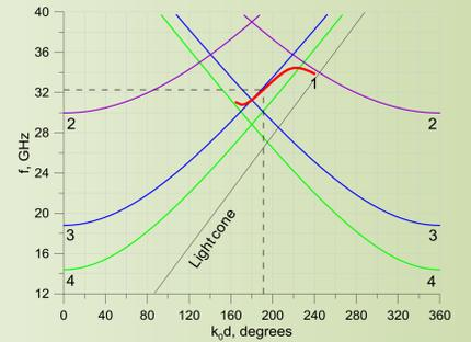
Dispersion of modes: 1 - TM<sub>01</sub>-TM<sub>11</sub> operating eigen wave, 2 - partial TM<sub>11</sub>, 3 - TM<sub>01</sub>, 4 - TE<sub>11</sub>
