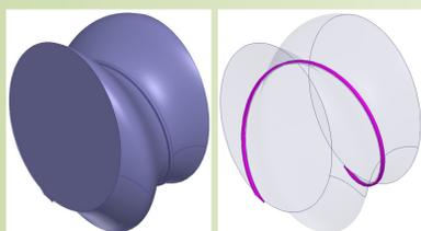
Groove with absorber is parallel to surface currents of operating eigen mode only
