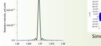
Spectrum of electron radiation with soft edge pulse
