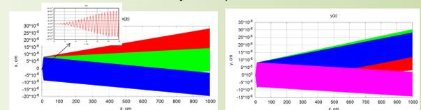
Simulation of electron trajectory in soft edge pulse with different injection phases
