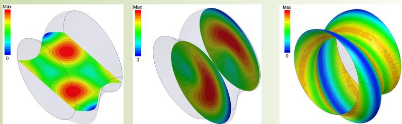
Module of electric field in middle plane, in two sequent cross-sections and on the surface.
