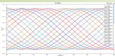
Accelerating field component vs longitudinal coordinate for different phases
