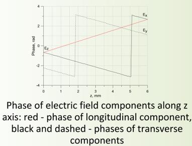
Phase of electric field components along z axis: red - phase of longitudinal component, black and dashed - phases of transverse components
