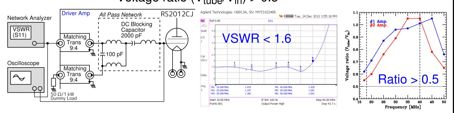
(b) Final amp.: Movable shorting plate of input stub was tuned so that input impedance is within an acceptable range (700 – 2000  $\Omega$ ).
