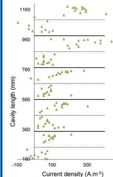
Figure 3: Current density distribution across an SPL 5 cell cavity from wall thickness measurements.
