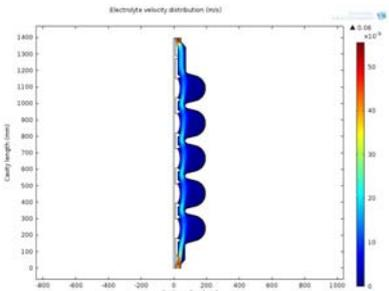
Figure 1: Electrolyte speed distribution in an axisymmetric cut of a SPL five cell cavity assembled with its cathode.
