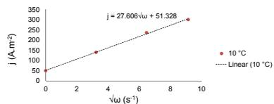
Figure 2: Experimental data acquired through the RDE shows the linear relation defined by the Levich equation between limiting current density and the square root of the angular velocity.
