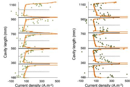
Figure 5: Current density distribution across the SPL five cell cavity for the first run. In green the experimental values and in orange the ones derived from the simulation data.
