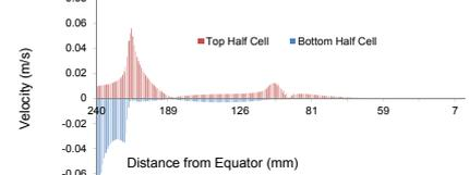
Figure 4: Electrolyte absolute velocity distribution at 5 mm from the cavity wall on a single cell. Negative velocity values are only for presentation purposes.
