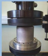
Brazed sample during shear test
