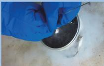
Brazed sample during thermal shock in N<sub>2</sub>
