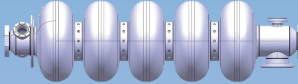
One of the main objectives of the SPL R&D effort at CERN is to develop 704 MHz bulk niobium  $\beta=1$  elliptical cavities operating at 2 K with an accelerating gradient of 25 MV/m and to test a string of four cavities in a cryo-module. The 5-cell cavities are made up of bulk niobium (RRR>300) and are equipped with SS flanges. The half-cells are shaped by spinning and assembled together with the cut-off tubes via EB welding
