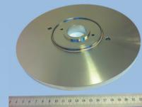
SS flange brazed to Nb tube with Cu as BFM
