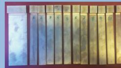
Brazing sample-test 2. SS plate brazed to SS plate with Cu as filler metal
