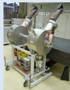
Left: Principle of slit-grid emittance measurement and specification of emittance-meter. Right: emittance-meter device.
