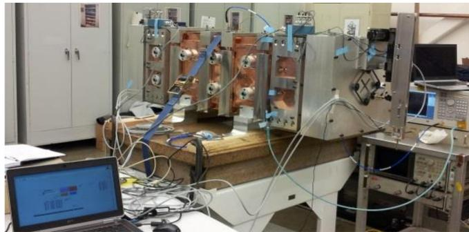
PXIE RFQ module 2 (out of 4 total) bead pull measurement set up at LBNL.
