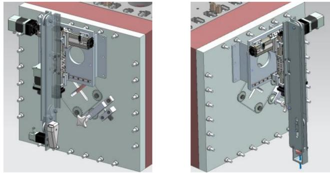
3D model of the bead pull system: motors and mechanical supports.
