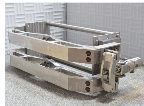
Figure 7. First prototype of the SSR1 double lever tuner.
