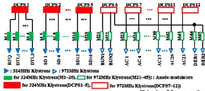
Configuration of klystrons and power supply system for klystrons in J-PARC 400MeV linac.
