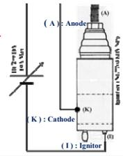
The cause of this decrease was taken to be the shaking sustained in the ignitrons during the earthquake, which resulted in the spillage of the mercury in the ignitrons onto the ignitrons. To repair the 24 faulty ignitrons, the method of impressing DC voltages (2-10 V) between the ignitrons (-) and the cathodes (+) was used. As a result of this treatment, 20 pieces were recovered (a recovery rate of 83.3%). The 4 remaining faulty ignitrons were replaced.
