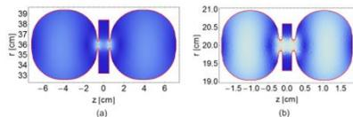
Fig. 5: S-band (a) and X-band (b) cavity FEM simulation, with plot of the electric field
