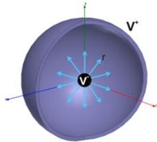
Fig. 1: Spherical cathode with natural expansion of electrons
