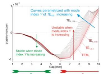
Fig. 4: Stability test in function of the cavity gap
