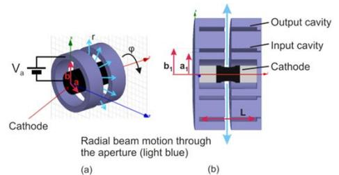
Fig. 2: Cylindrical cathode with radial expansion of electrons (a), Cylindrical klystron with two coaxial resonators (b)
