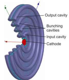
Fig. 7: Overview of the cylindrical klystron
