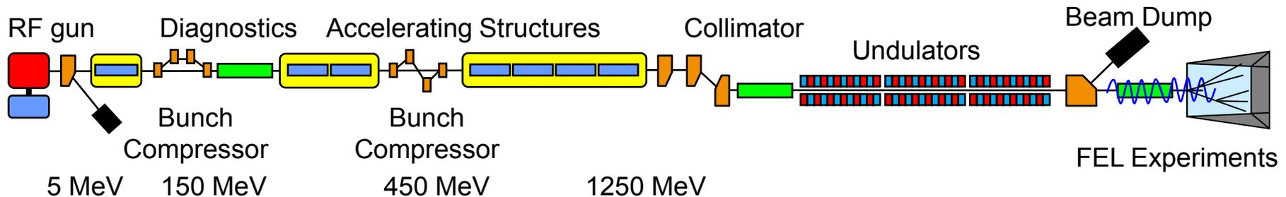
→ electron source has to produce lowest possible emittance !!
