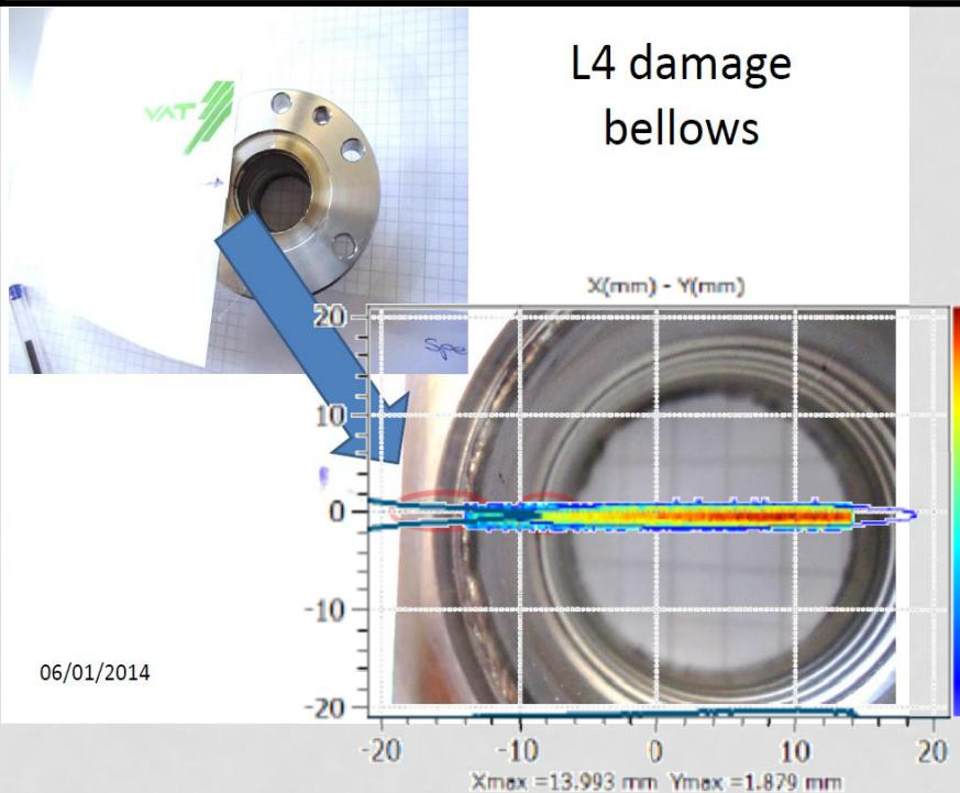
**A severe misalignment** between the RFQ and the MEBT that was not present at the 3 MeV test stand and was later confirmed by survey
