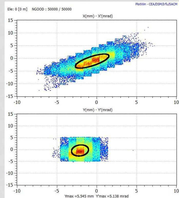
Emittance measured with chopper off (left) and with chopper on (right) downstream the inline dump
