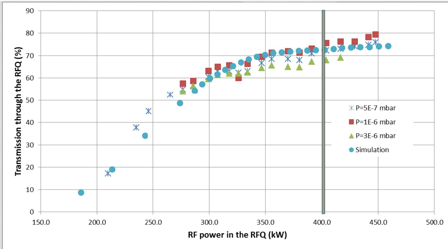
RFQ Transmission vs. RF power for different pressure in the LEBT (neutralisation). The nominal RFQ power is 400 kW.
