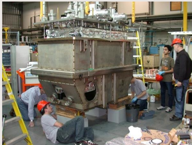
Top assembly into tank
