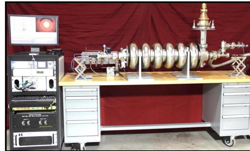
6 cell HB cavity on plasma processing station
