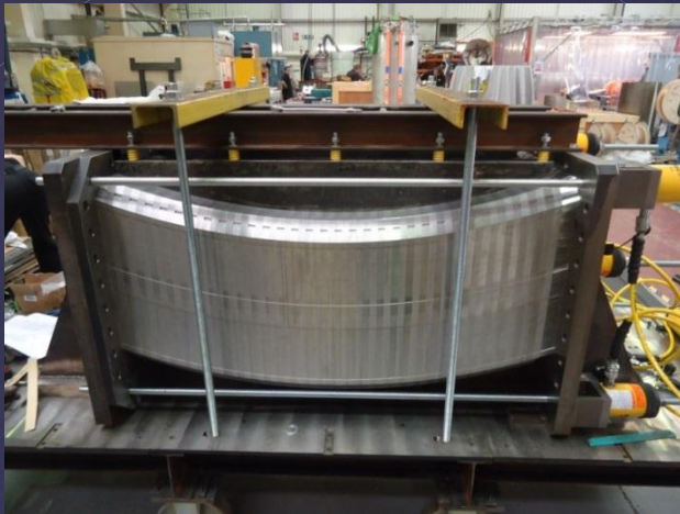
Pre-series dipole yoke stacking
