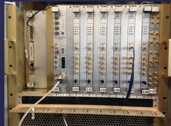
LLRF system for a complete cryomodule (6 cavities)
