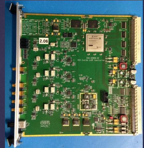
LLRF system for a complete cryomodule (6 cavities)
