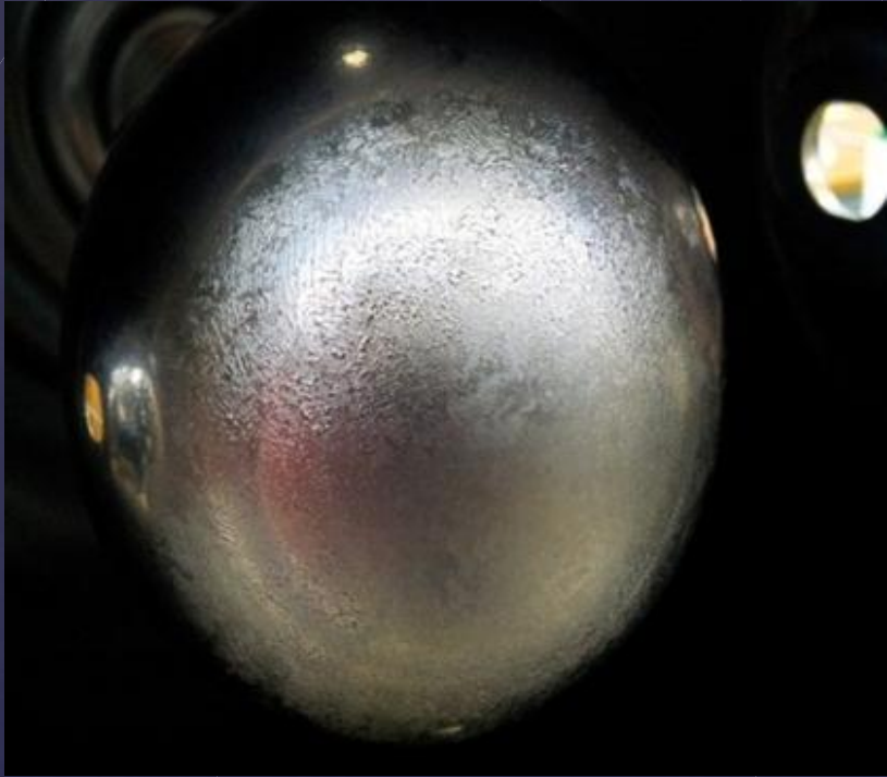
Central electrode: 20 mm diameter, at earth potential
