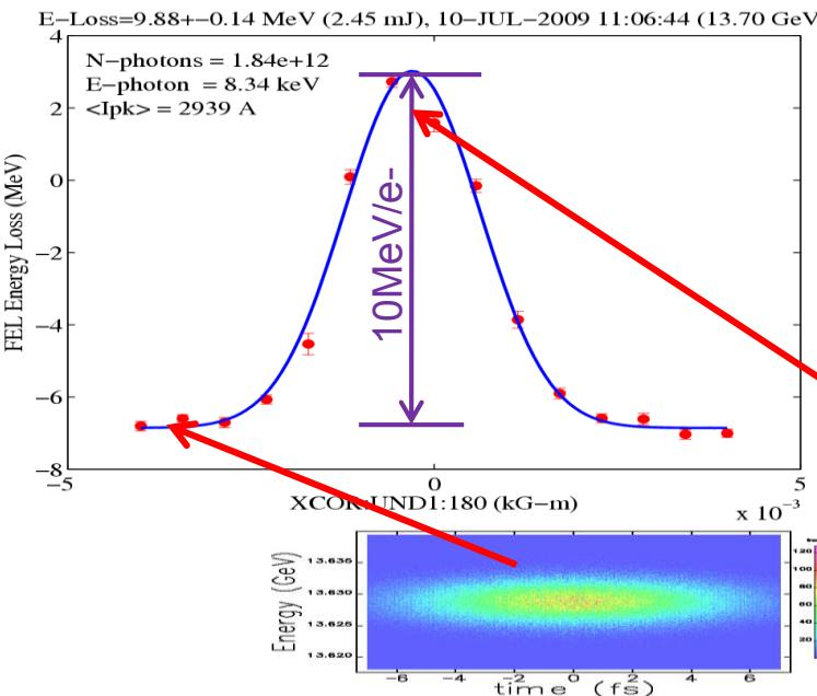
→ to measure the **time-resolved** lasing effect (“footprint”) left on the electron bunch.
