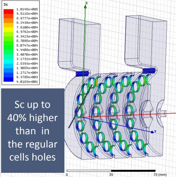
By reducing the coupling holes radius closer to the coupling slot the problem is solved
