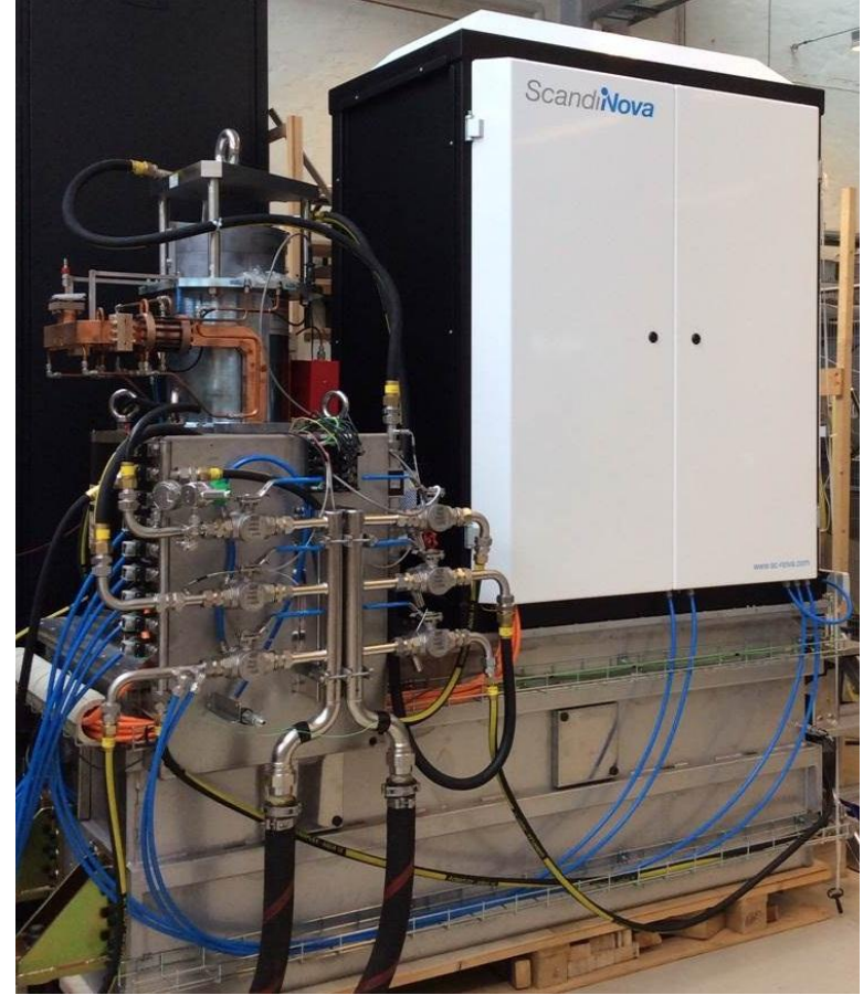
50MW Klystron and K2-3 Modulator
