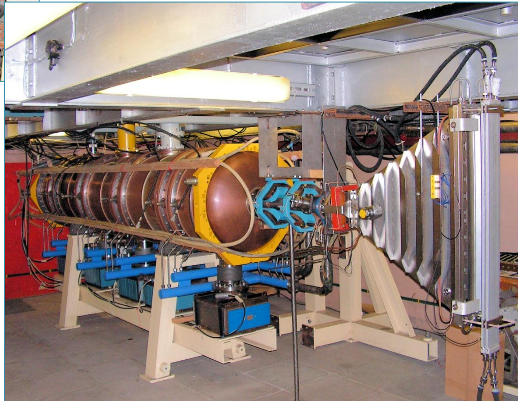
Accelerating structure with beam scanning system
