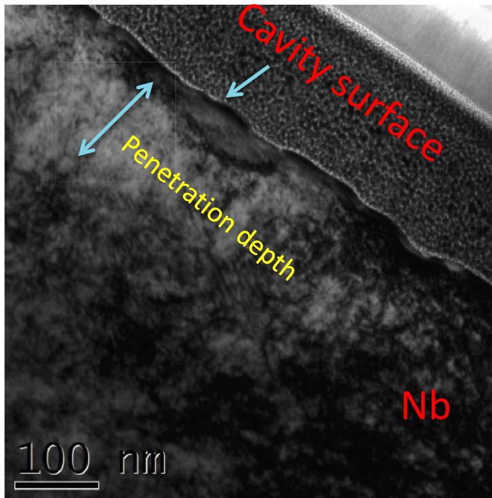
Electron diffraction patterns from the penetration depth taken at 94K reveal the difference
