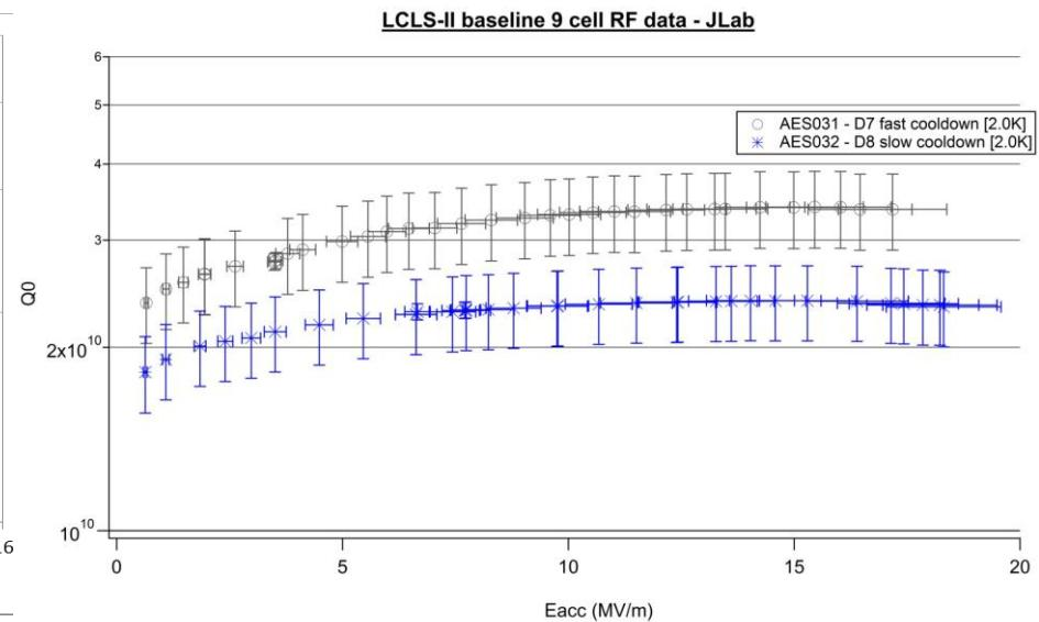
JLab VTS data on a 9-cell
