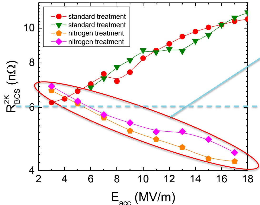
Anti-Q-slope emerges from the BCS surface resistance decreasing with field
