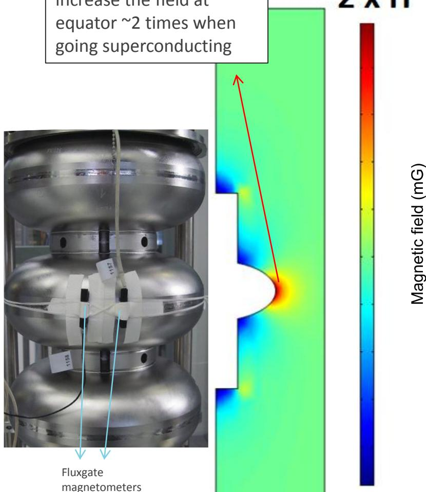
It turns out the expulsion efficiency can be controlled by the cooldown procedure through  $T_c=9.2K$  (fast/slow, uniform or not)
