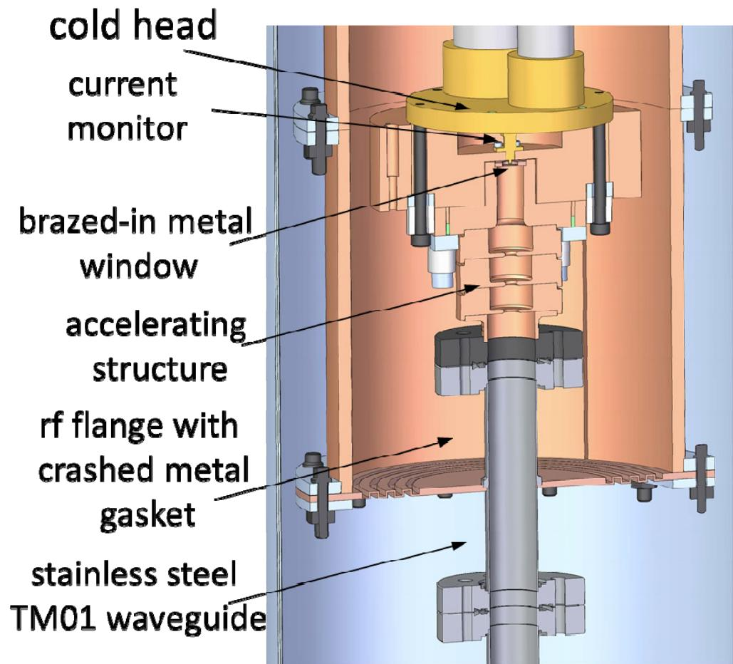
Structure is running now at an *accelerating gradient of 240 MV/m @ 45 K*
