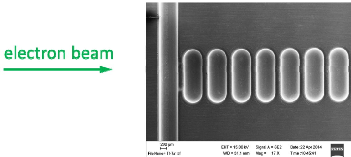
Input coupler, cells 1-7, no damage
