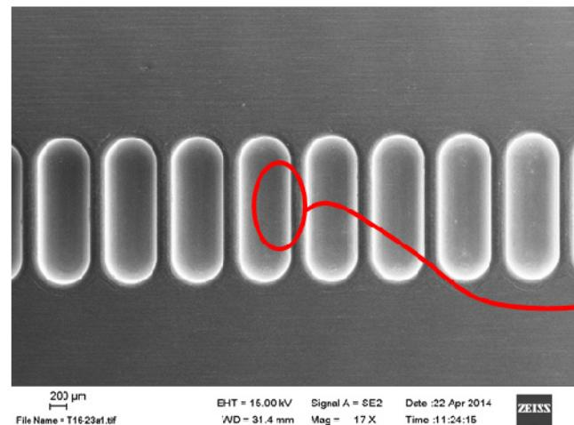
Cells 16-23, fist signs of damage
