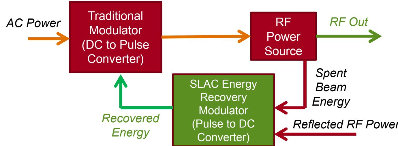
Feed-forward energy recovery modulator technology enables traditionally wasted energy to be utilized on subsequent pulses
