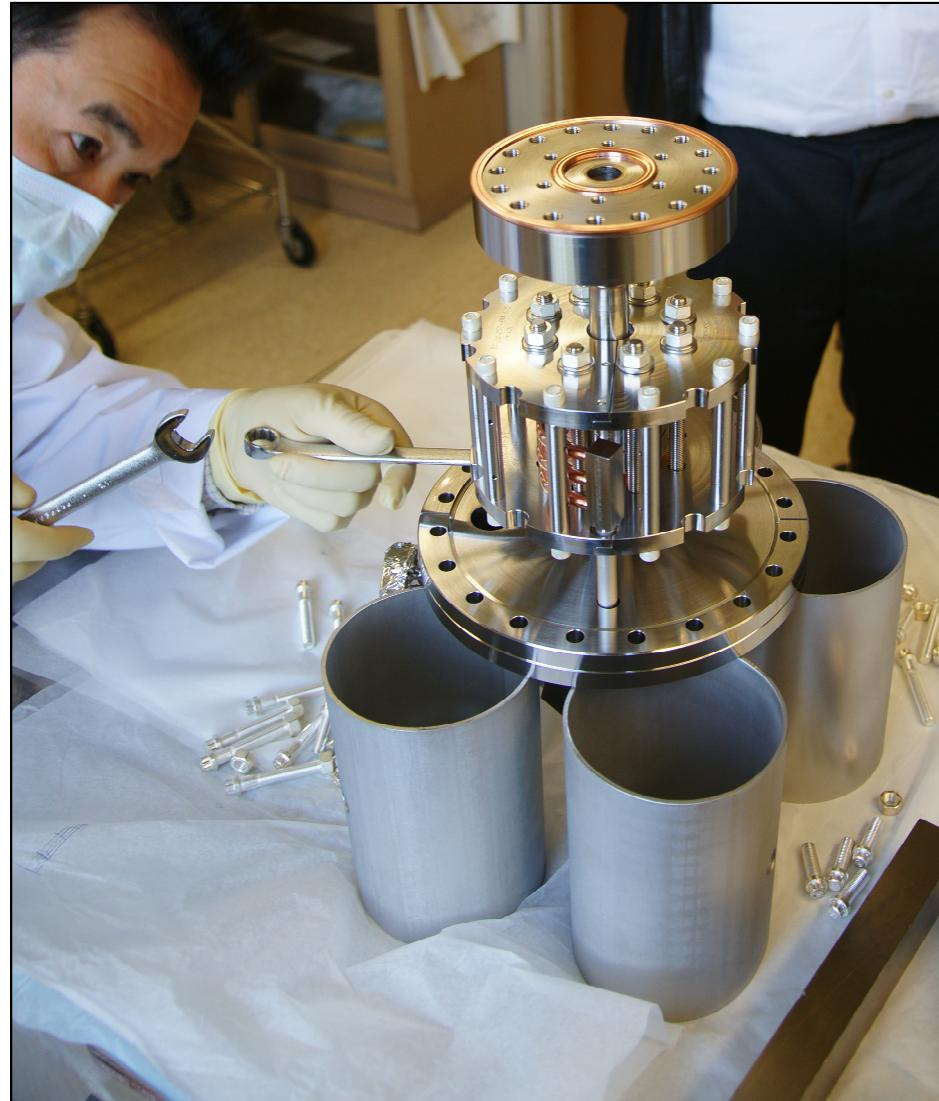
Clamped structure for testing without brazing
