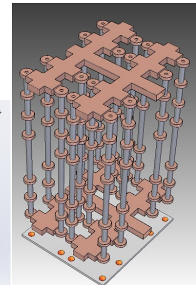
Multi-beam klystron assembly
