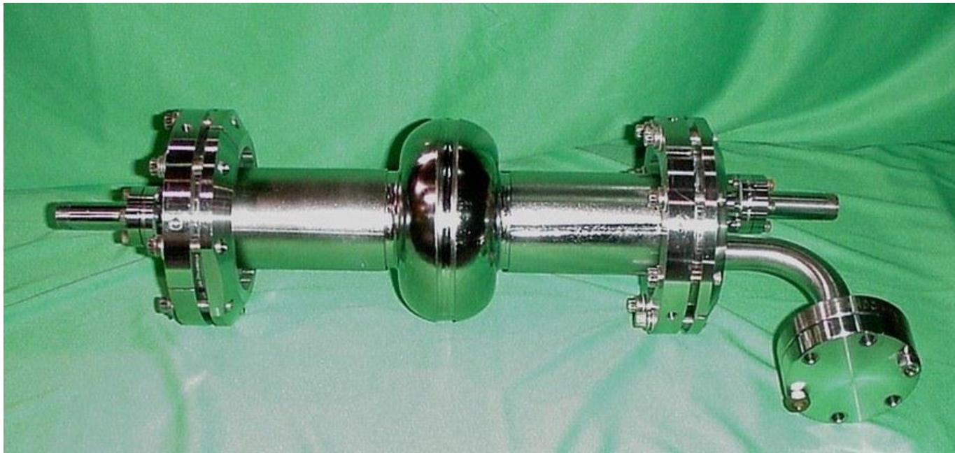
**Demonstration of CW 2.45 GHz magnetron driving a specially manufactured superconducting cavity in a vertical test facility at JLab and the control of phase in the presence of microphonics was successful.**
