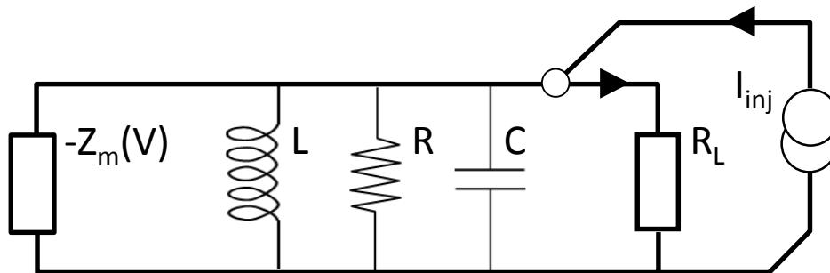
**Negative impedance  $-Z_m$  to represent magnetron spokes excitation of RF in anode.**
