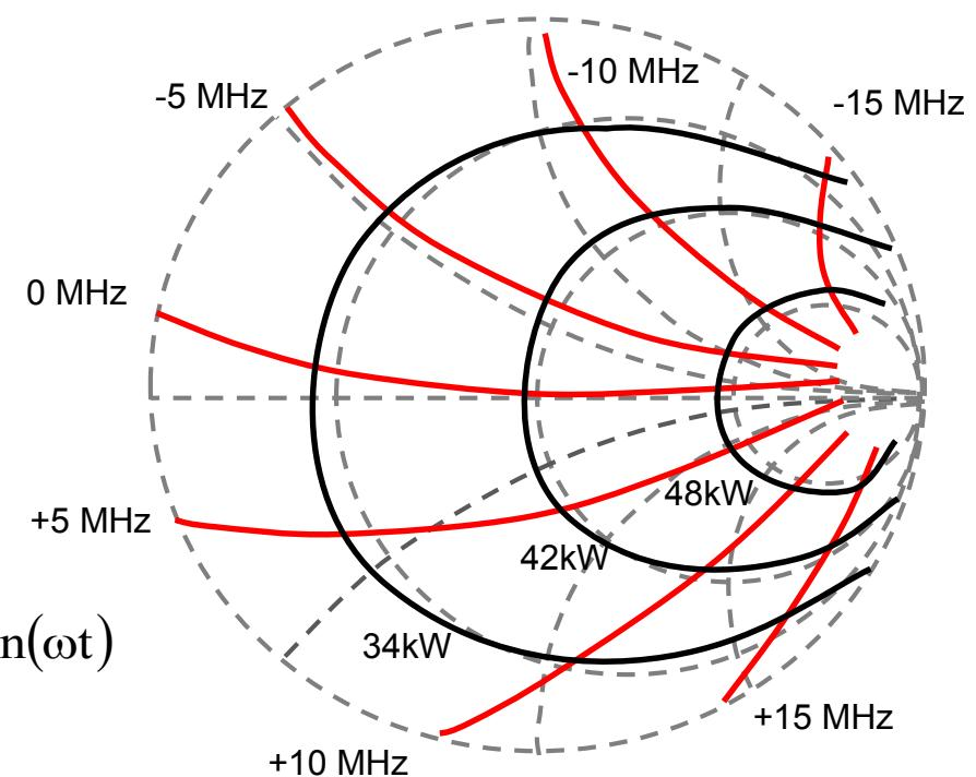
**Rieke diagram plots constant frequency and constant power lines on an admittance chart**
