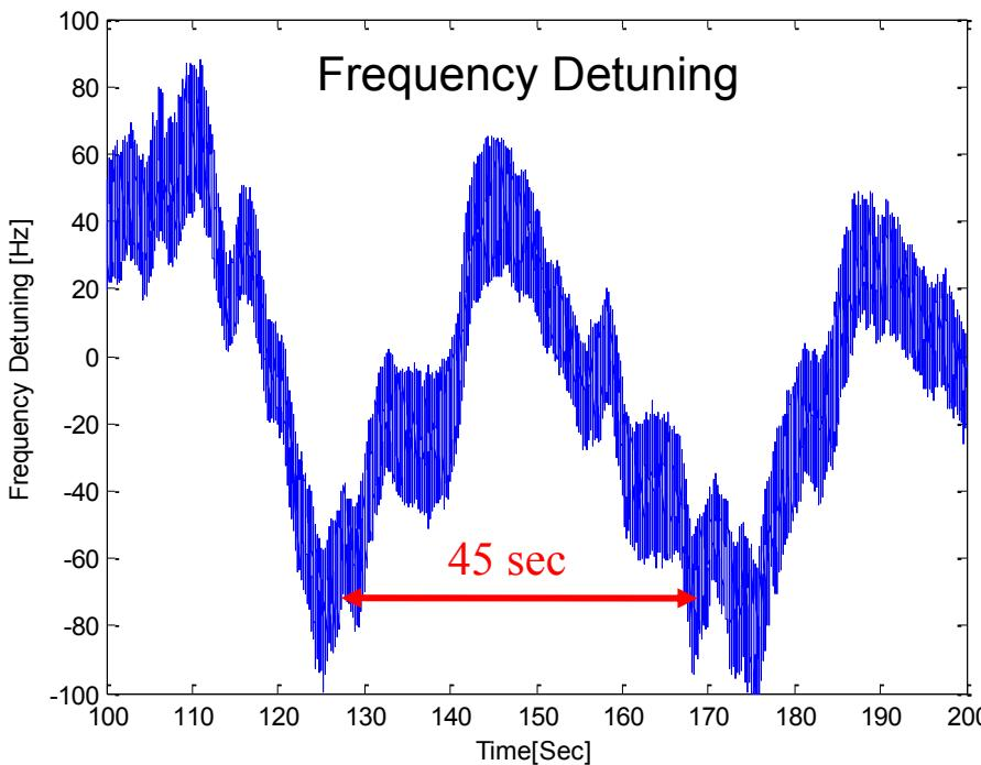
**Suggested solution** - Increase the rigidity of the tuning fog and add ribs at the vicinity of the beam line. This should reduce the sensitivity of the HWR to helium pressure by a factor of  $\sim 3$ .
