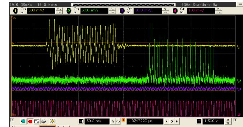
Minimum chopper pulse length of 160 ns as measured by BPM and a FFC
