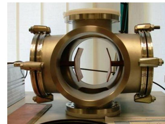
The deflecting electrodes inside the beam line
