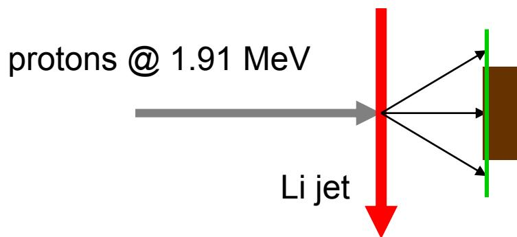
creates in lab stellar neutron spectra with  $T=300$  million degrees  $\sim kT = 25 \text{ keV}$  neutron flux approaching  $\sim 10^{11} \text{ n/sec}$
