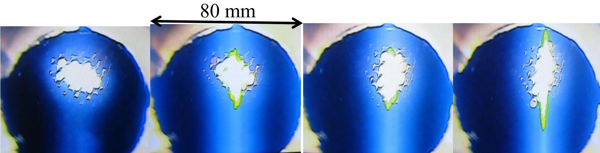
Varying quads while observing 0.3 mA beam (0.65 kW)
