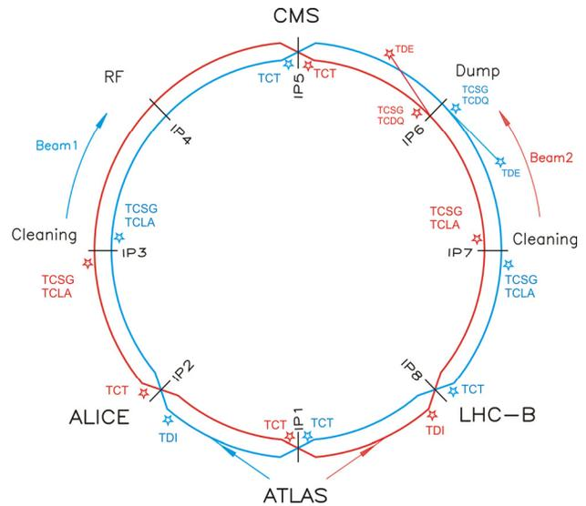
Figure 1: Location of beam stops during injection tests.
