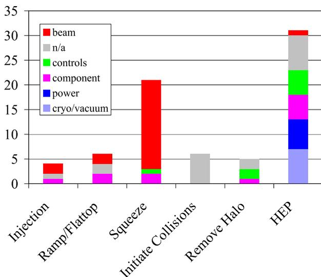
Figure 1: Occurrence of quenches over the Tevatron collider cycle.
