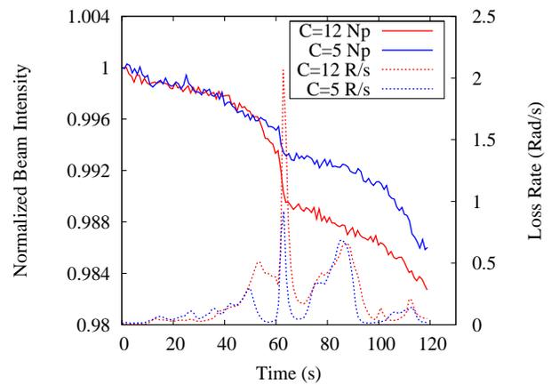
Figure 5: Comparison of proton intensity and loss rates in the low-beta squeeze before and after chromaticity change. Step 14 is at 60 s.
