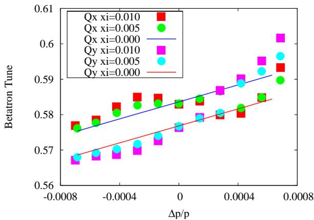
Figure 3: Tunes vs. momentum deviation for different values of beam-beam parameter.
