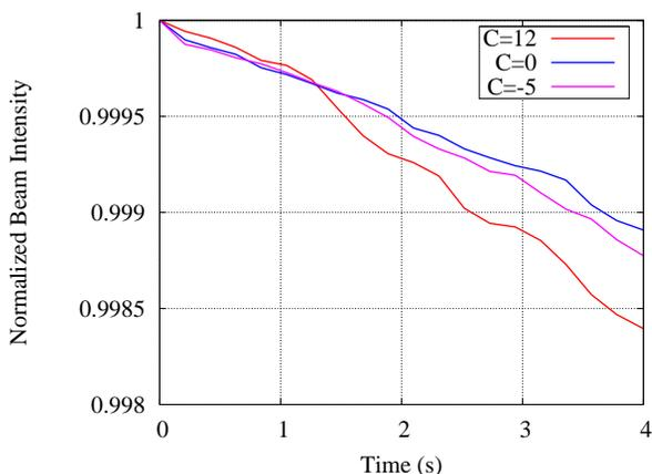
Figure 4: Beam loss at low beta step 14 vs. chromaticity.
