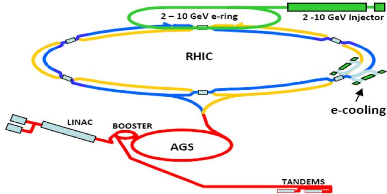
Figure 2: Schematic layout of the eRHIC ring-ring electron-ion collider [4].
