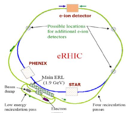
Figure 6: Schematic layout of the eRHIC linac-ring electron-ion collider [4].
