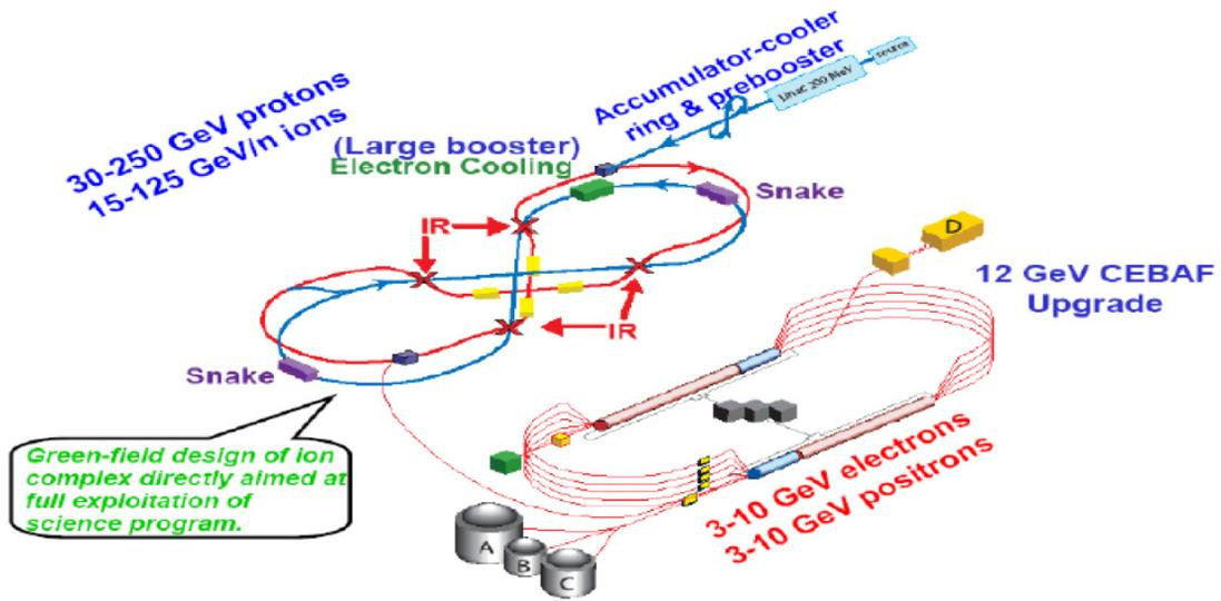
Figure 3: Schematic layout of the ELIC ring-ring electron-ion collider [3].
