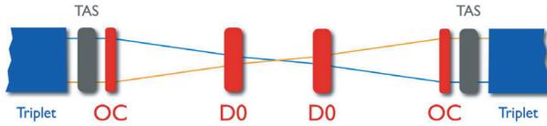
Figure 4: Layout of early separation scheme [7].
