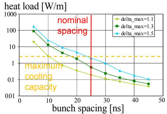
Figure 1: Simulated electron-cloud heat load per unit length for the LHC arc, assuming nominal bunch charge  $N_p = 1.15 \times 10^{11}$  and 50% probability of elastic scattering for low-energy electrons; the three curves correspond to three values of  $\delta_{\max}$  [4].
