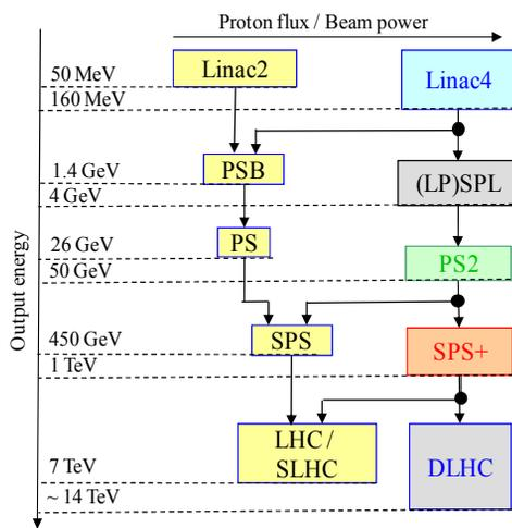
Figure 7: CERN accelerator-complex upgrade plan [23].
