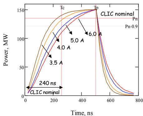
Figure 6: Expected power at several train currents as a function of the pulse length.
