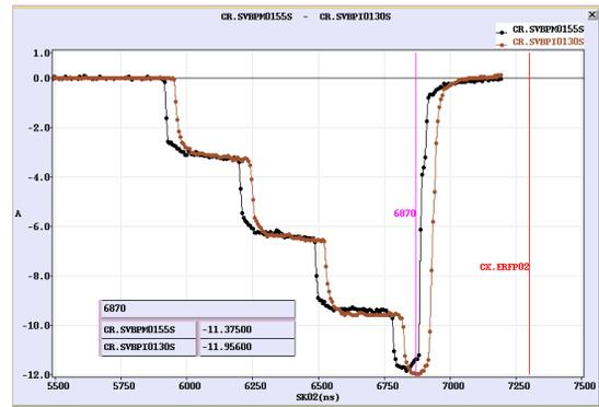
Figure 5: Factor 4 recombination in the CR. The beam current in the first two BPMs is shown.
