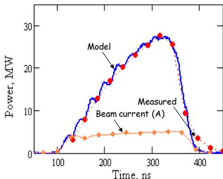
Figure 7: Comparison between the measured and the expected power.
