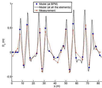
Figure 3: Comparison between the predicted and the measured dispersion in the CR.
