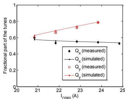
Figure 4: Comparison between the predicted and the measured horizontal and vertical tune.
