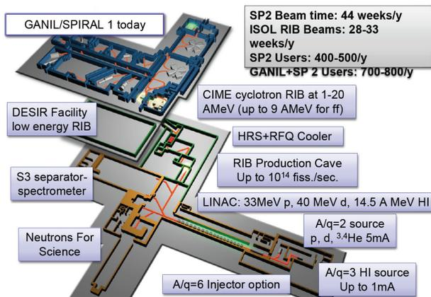
Figure 1: New and existing (in dark blue) facilities at GANIL site. Accelerator and stable beam physics in brown, RIB in green.
